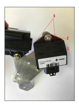
Take ECU (1) and fix it on the mounting plate by using a rubber buffer M6, distance sleeve, washer and lock nut M6 (2).
