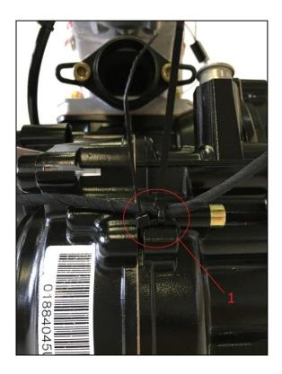
Fix the cable of shift contact on the threat of the engine housing (1)
