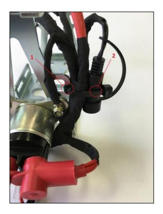
Take one tie wrap large and fix the harness on the battery frame (1)
