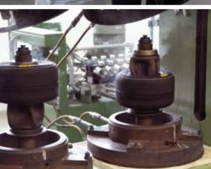
Above, different phases of Mojo manufacturing process by German tyre manufacturer Heidenau, one of which stamps a barcode on each tyre to make it identifiable through the digital Tyre Tracking System (TTS). The TTS is not only a tool for quality assurance, but also eases the distribution and the handling of tyres at the track.
